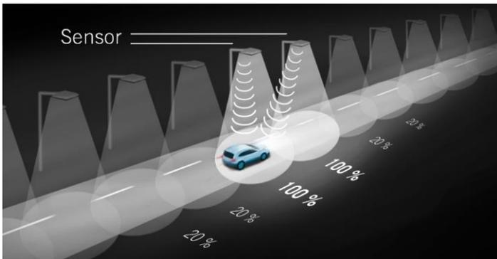
This solution does not only work with rigid dimming profiles, furthermore it is possible to react to the real traffic by detecting the motion. The main application areas are parks, parking spaces, cycle paths, roundabouts and ring roads.
